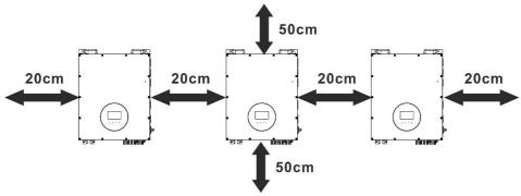
**NOTE:** For proper air circulation to dissipate heat, it's necessary to allow a clearance of approx. 50 cm to the side and approx. 20 cm above and below the unit. Be sure to install each unit in the same level.
