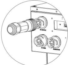
**CAUTION:** It's only allowed to connect load to "AC Output Connector". Do NOT connect the utility to "AC Output Connector".
