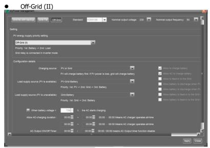
PV energy supply priority setting: 1st Battery, 2nd Load
