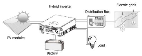
Figure 1 Basic hybrid PV System Overview
