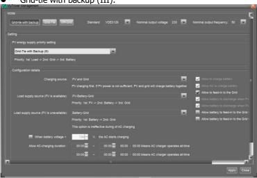
PV energy supply priority setting: 1st Load, 2nd Grid and 3rd Battery
