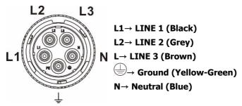
The reference tightening torque is 4-5 N.m.
