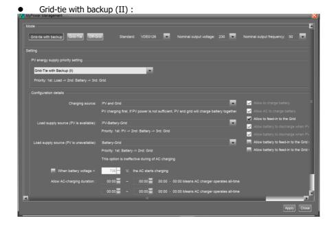
PV energy supply priority setting: 1<sup>st</sup> Load, 2<sup>nd</sup> Battery and 3<sup>rd</sup> Grid.
