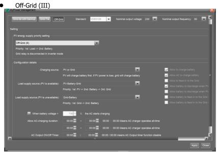
PV energy supply priority setting: 1st Load, 2nd Battery
