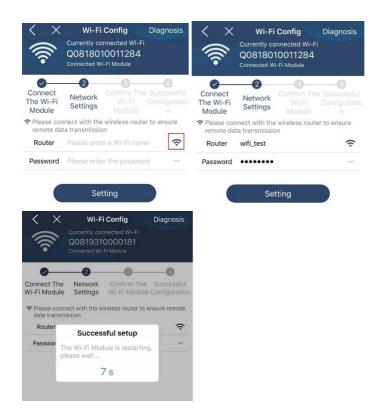
Step 4: Tap "Confirm" to complete the Wi-Fi configuration between the Wi-Fi module and the Internet.
