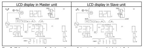
Step 5: If there is no more fault alarm, the parallel system is completely installed. Step 6: Please switch on all breakers of Line wires in load side. This system will start to provide power to the load.
