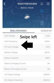
**[Basic Information]** displays basic information of the inverter, including AC voltage, AC frequency, PV input voltage, Battery voltage, Battery capacity, Charging current, Output voltage, Output frequency, Output apparent power, Output active power and Load percent. Please slide up to see more basic information.
